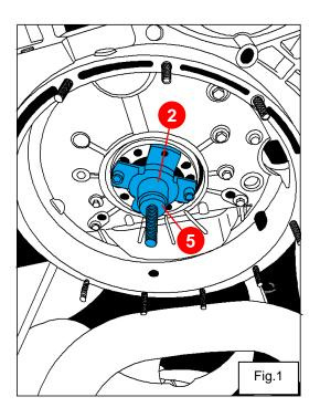
Step 1: Refer to Fig.1 Install no.2. Depend on the size, take no.6 or no.7 to screw on no.2. Then install no.5
