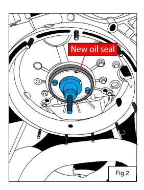
Step 2: Refer to Fig.2 Put on the new oil seal.
