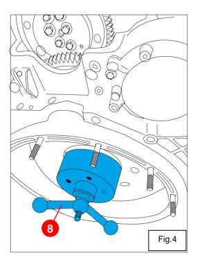
Step 4: Refer to Fig.4 Install no.8, spin the handle to an appropriate place. Then finish installing.
