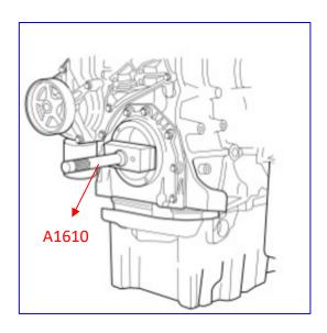
If you don't use special tool to install oil seal. It might causing oil seal bad install and leak oil. Then you will need to extract and install the part again. This tool can make installing quickly and easily.
