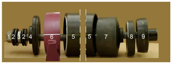
The centering ring of the receiver tube is used to center the receiver tube on the trailing arm receptacle. When the installation tool is used, the centering ring must always be positioned against the trailing arm receptacle.
